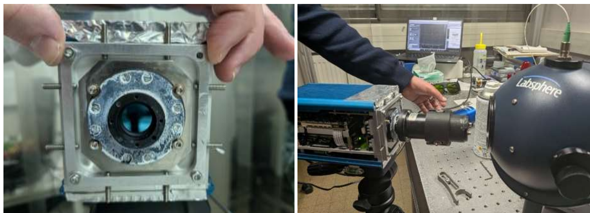
Figure 15: Integration of NanoCarb-P CO2 camera: left: alignment of the interferometric core regarding the detector and right: experimental setup for the alignment
