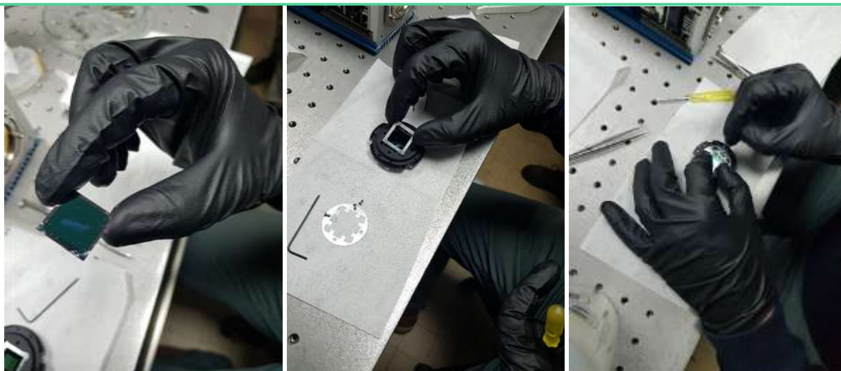
Figure 14: Integration of NanoCarb-P CO2 camera: mounting the interferometric core and Left: coated CO2 interferometric plate.
